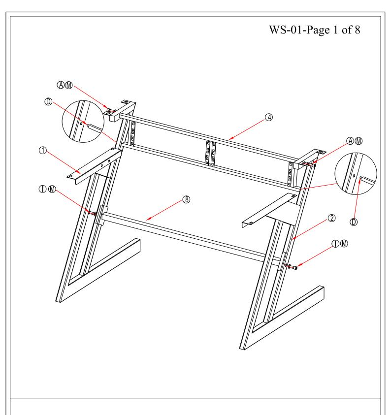
1.Using the allen key bolts and washers to connect two legs with the cross bar and equipment rack as he picture showed.
