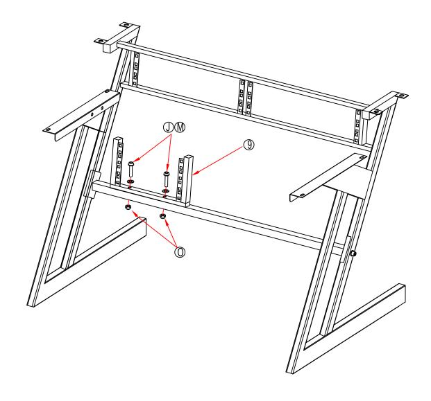
2. Put the 4U rack on the cross bar and tighten the screws.
