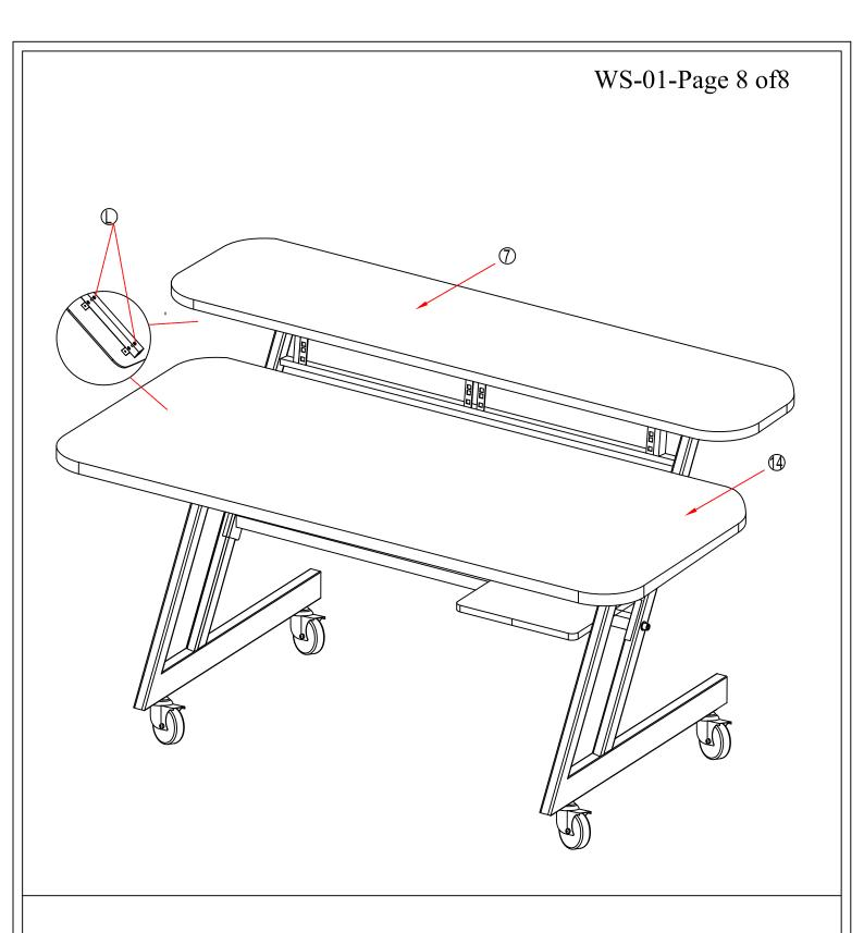
8. Mount the center shelf and top shelf on support brackets at desired depth with provided wood screws.
