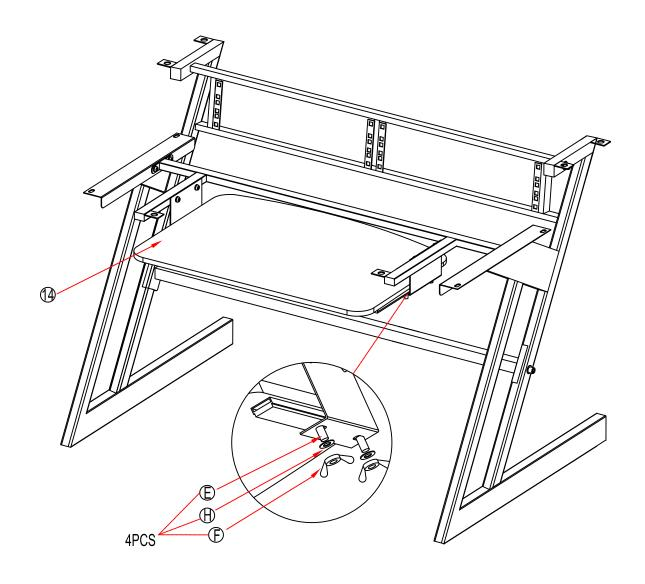
4. Mount the keyboard shelf on the keyboard shelf brackets and tighten the screws.
