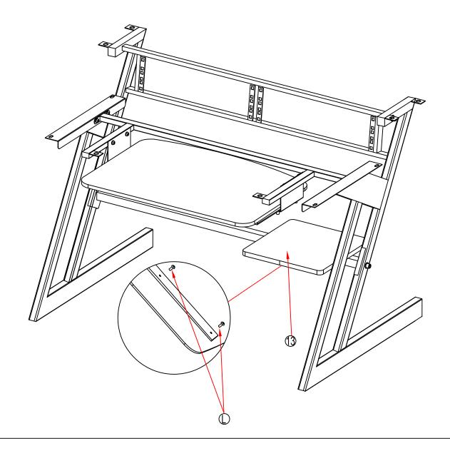
6. Attach lower shelf onto the brackets.
