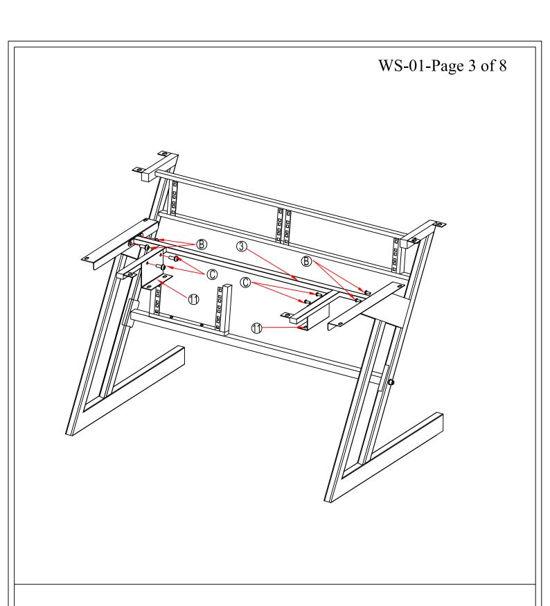
3.Attach keyboard shelf support bracket as above picture and tighten the bolts.
