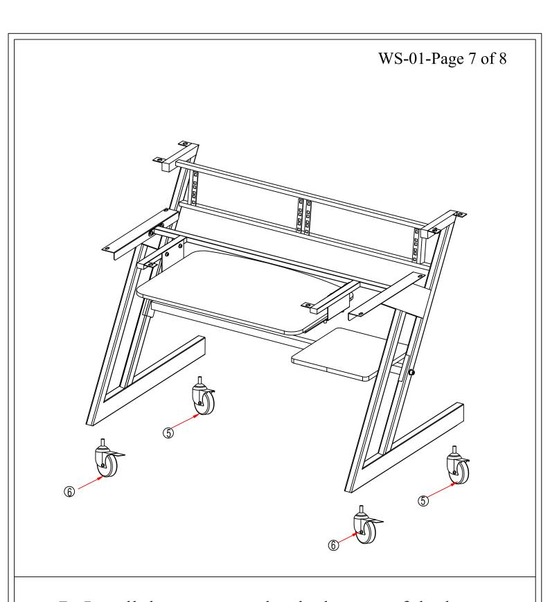
7. Install the casters under the bottom of the legs (two lockable ones in front, while the others in back)
